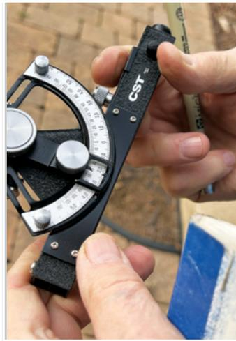
Jim Bagley uses an inclinometer to measure tree heights.
